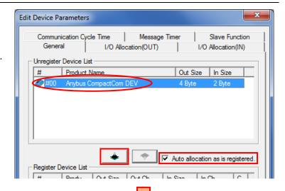
The Robot (#00) is registered in the *Register Device List* Field.
